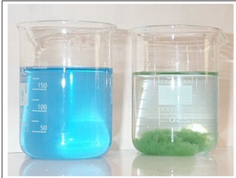
Picture from treatment of rinse water after copper alkali etch process with SCANPOL® 27
